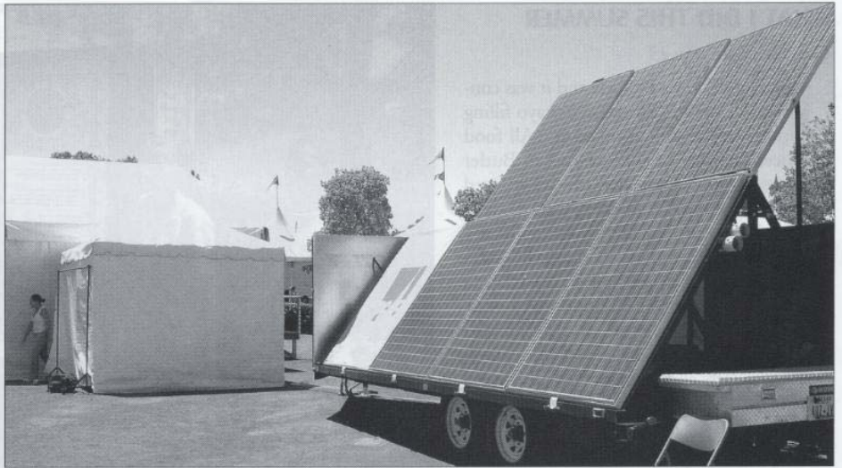
The mobile solar array provided power for sound and light at the Ben & Jerry’s stage and was sponsored by PG&E.
